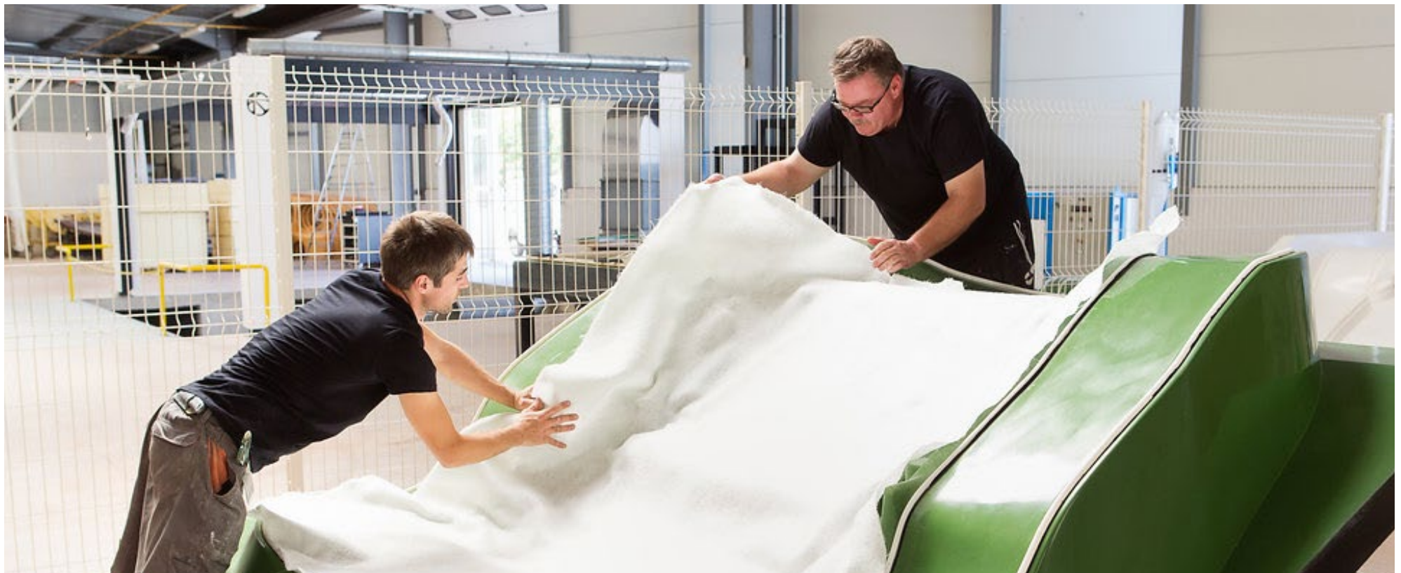
Loading of body panels by hand
